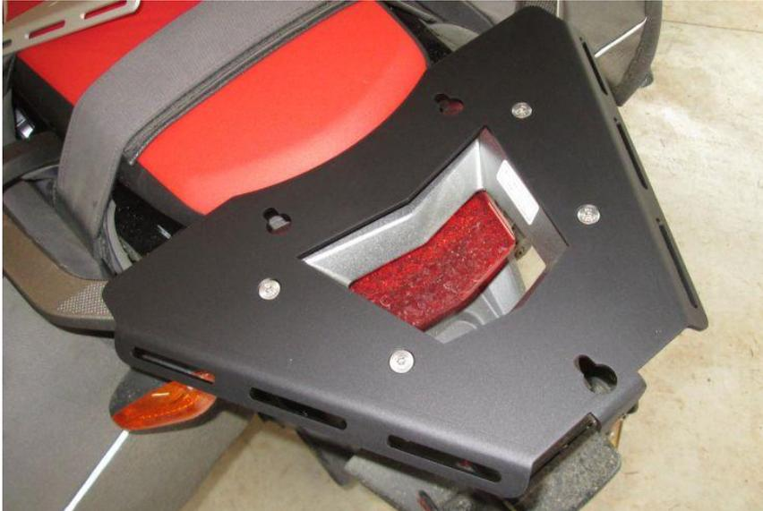
14. From under the underside of the rack place the M6 fender washers (#3) and locknuts (#4) on the screws and tighten them.
