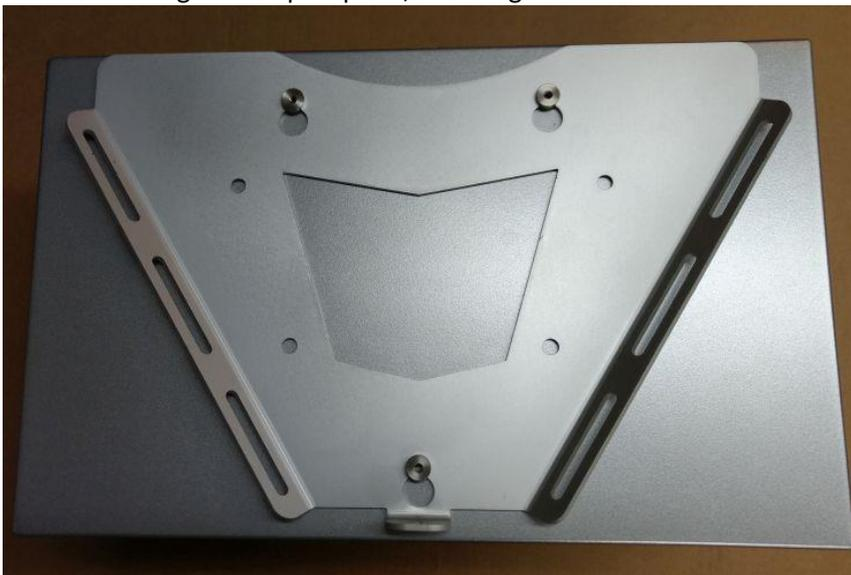
6. Take a sharpened pencil or a 3mm (1/8") drill bit and mark the center of the pucks through the holes onto the top case. Make sure you don't move the adapter plate in the process.
